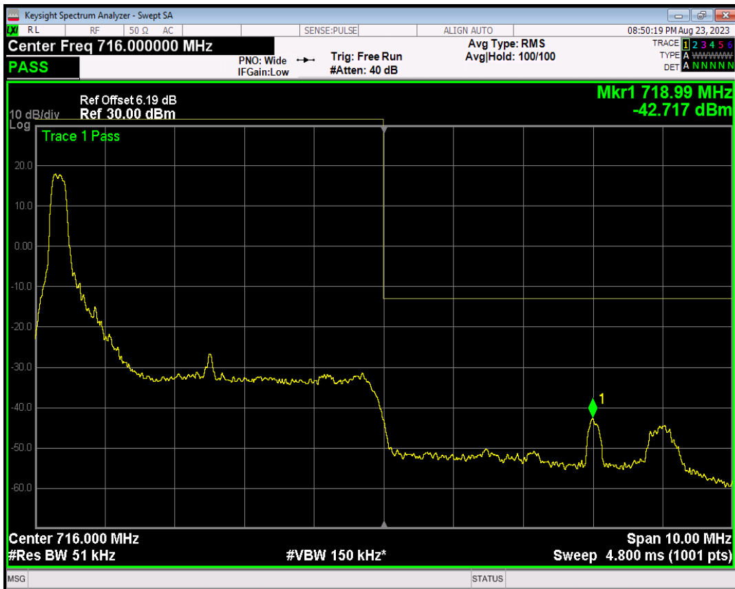
Band17 16QAM BW=5MHz Channel=23825 RB Size=1 Position=#Max
