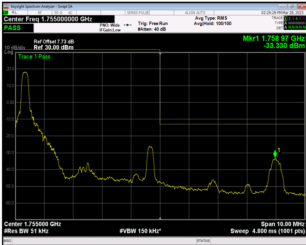
Band4 QPSK BW=5MHz Channel=20375 RB Size=1 Position=#Max
