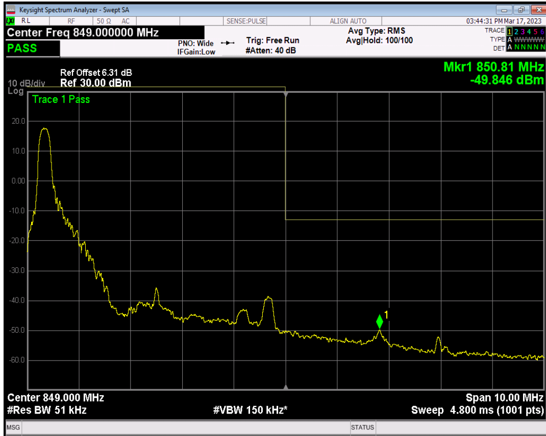
Band26(824-849) QPSK BW=5MHz Channel=27015 RB Size=1 Position=#Max
