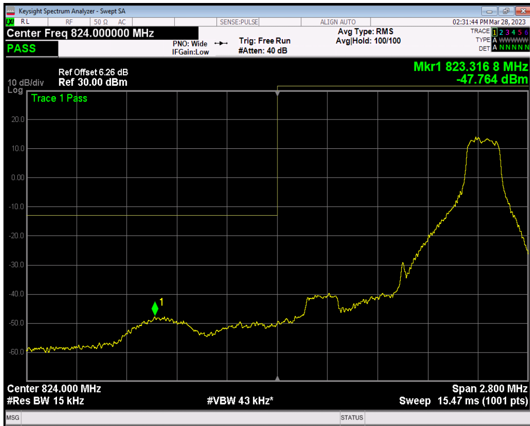
Band5 QPSK BW=1.4MHz Channel=20407 RB Size=6 Position=#0
