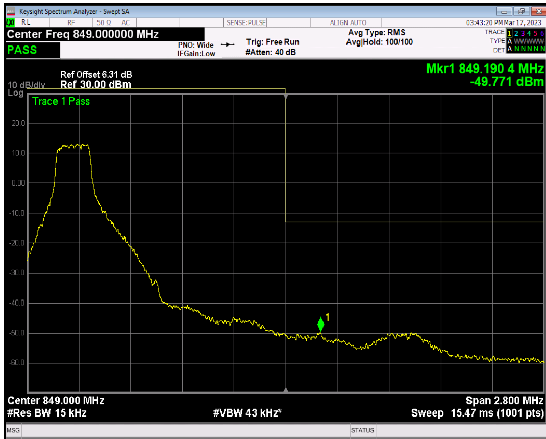
Band26(824-849) QPSK BW=1.4MHz Channel=27033 RB Size=1 Position=#Max
