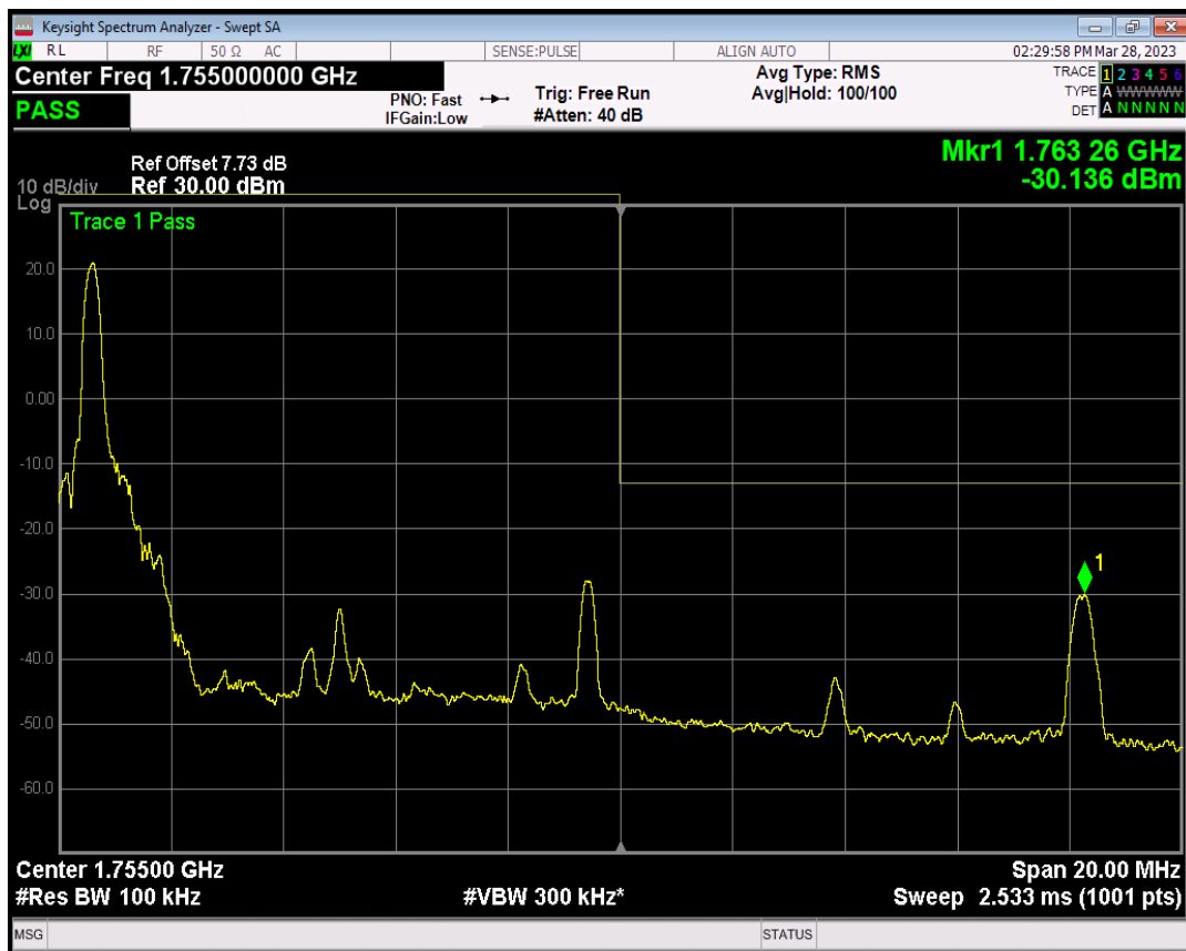
Band4 QPSK BW=10MHz Channel=20350 RB Size=1 Position=#Max
