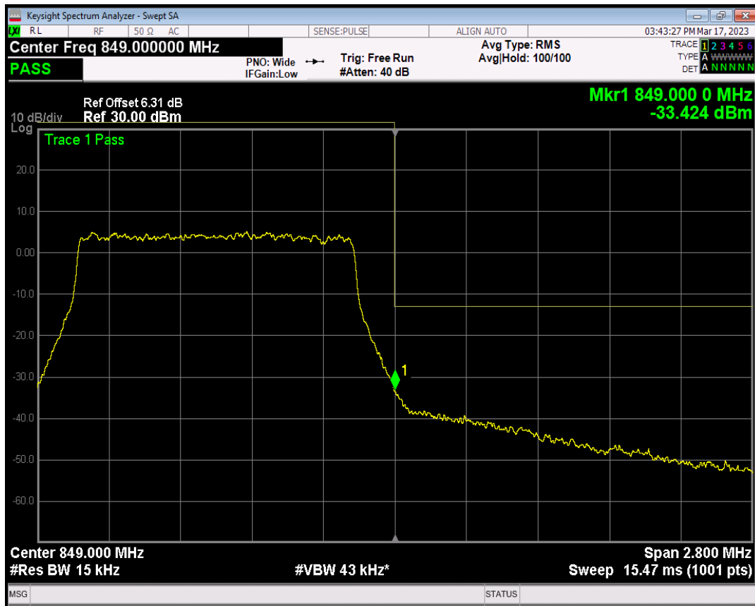
Band26(824-849) QPSK BW=10MHz Channel=26840 RB Size=1 Position=#0
