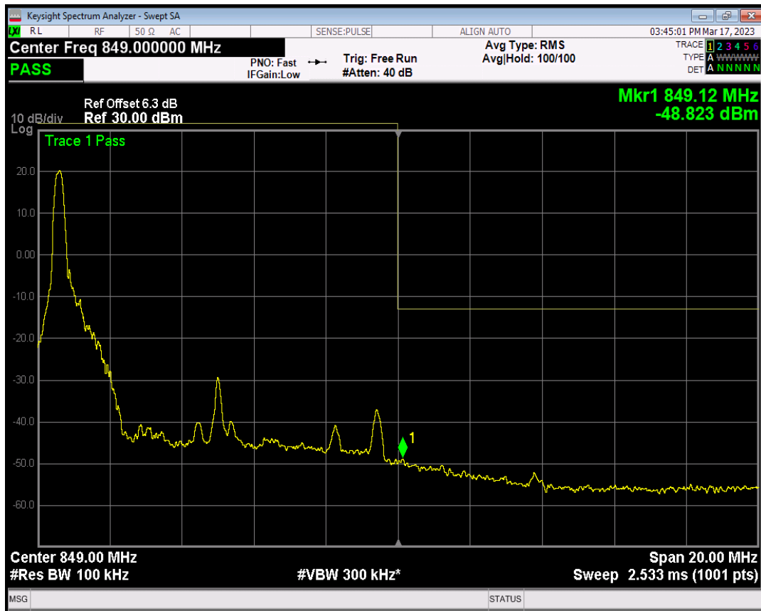
Band26(824-849) QPSK BW=10MHz Channel=26990 RB Size=1 Position=#Max
