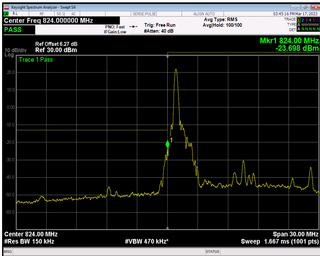
Band26(824-849) QPSK BW=15MHz Channel=26865 RB Size=1 Position=#Max
