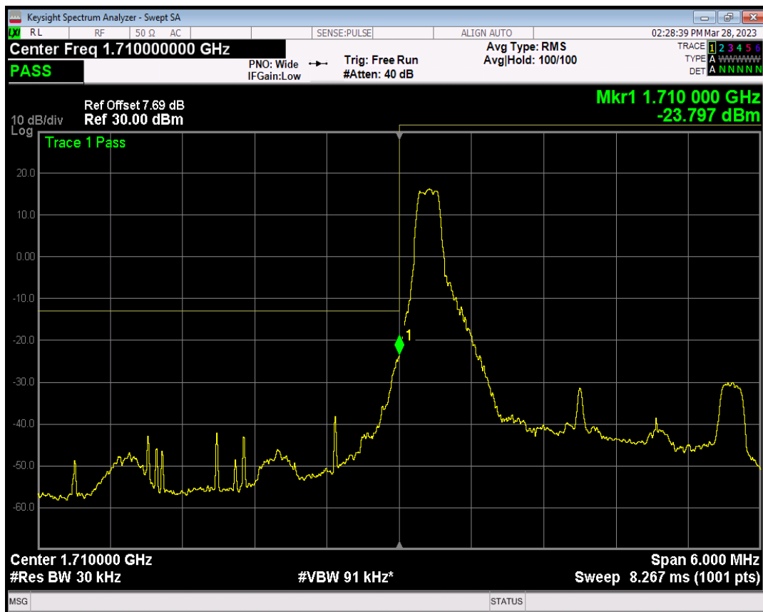
Band4 QPSK BW=3MHz Channel=19965 RB Size=1 Position=#Max
