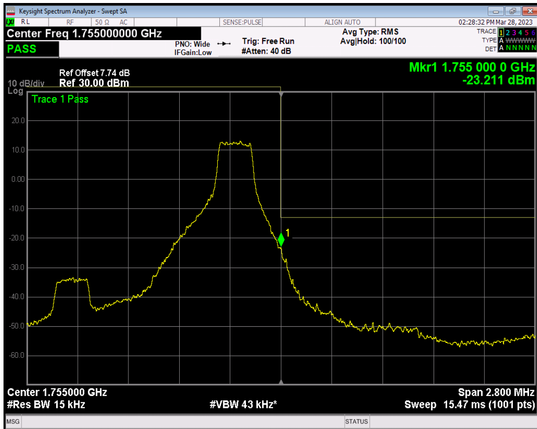
Band4 QAM16 BW=1.4MHz Channel=20393 RB Size=6 Position=#0
