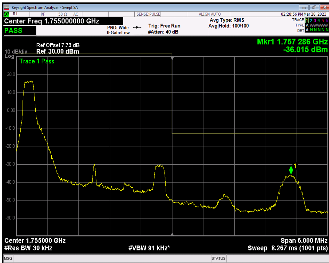
Band4 QPSK BW=3MHz Channel=20385 RB Size=1 Position=#Max
