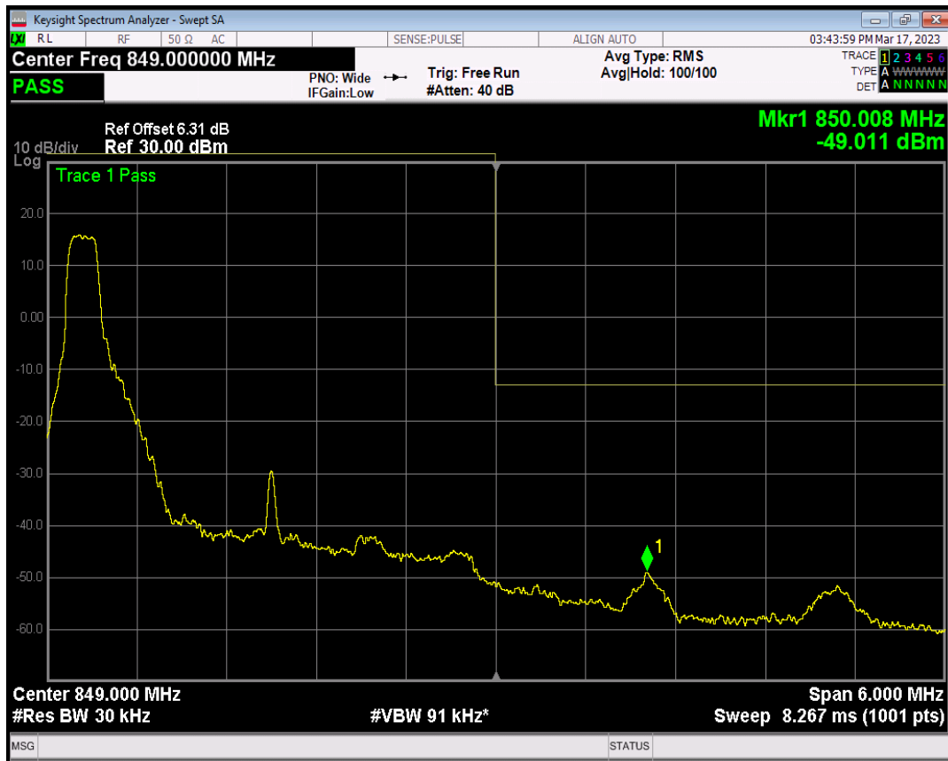
Band26(824-849) QPSK BW=3MHz Channel=27025 RB Size=1 Position=#Max
