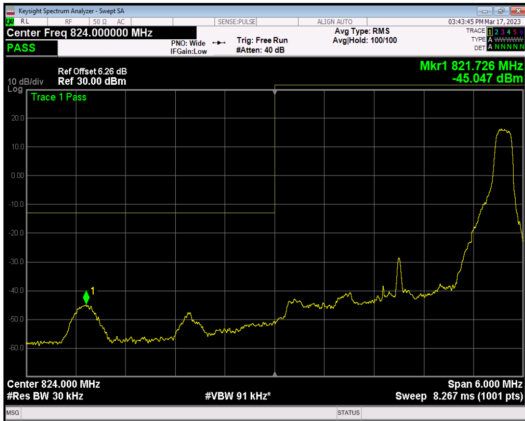
Band26(824-849) QPSK BW=3MHz Channel=26805 RB Size=15 Position=#0
