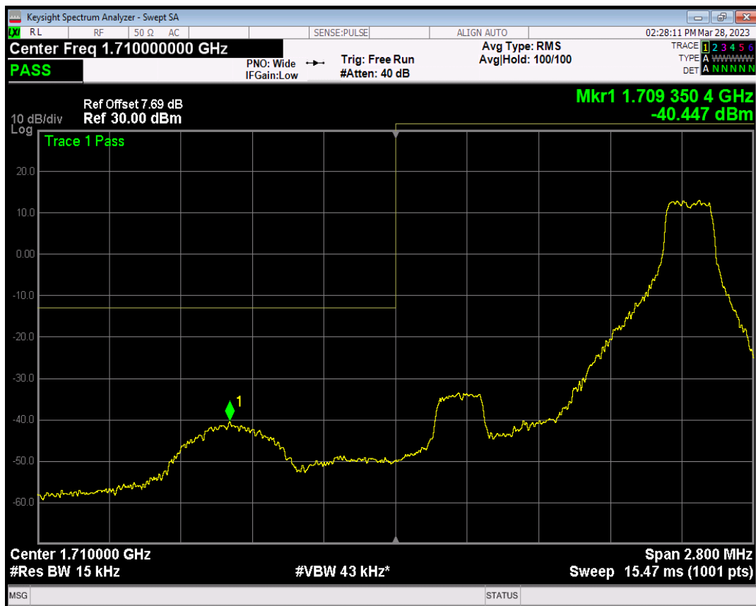
Band4 QAM16 BW=1.4MHz Channel=19957 RB Size=6 Position=#0
