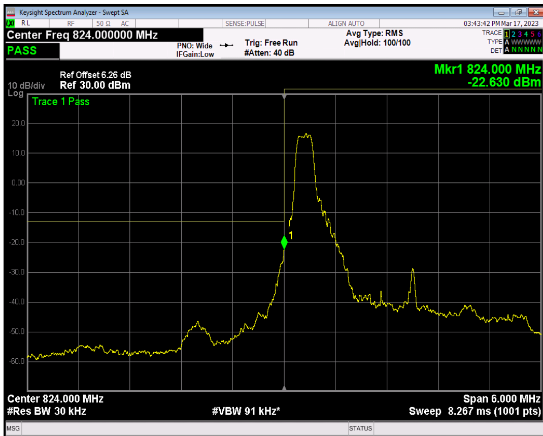
Band26(824-849) QPSK BW=3MHz Channel=26805 RB Size=1 Position=#Max
