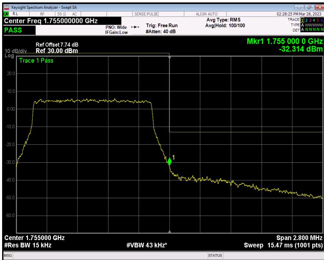
Band4 QAM16 BW=1.4MHz Channel=20393 RB Size=1 Position=#0
