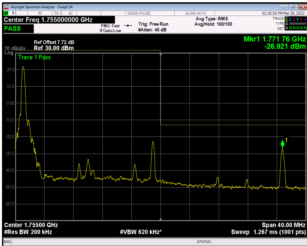
Band4 QPSK BW=20MHz Channel=20300 RB Size=1 Position=#Max
