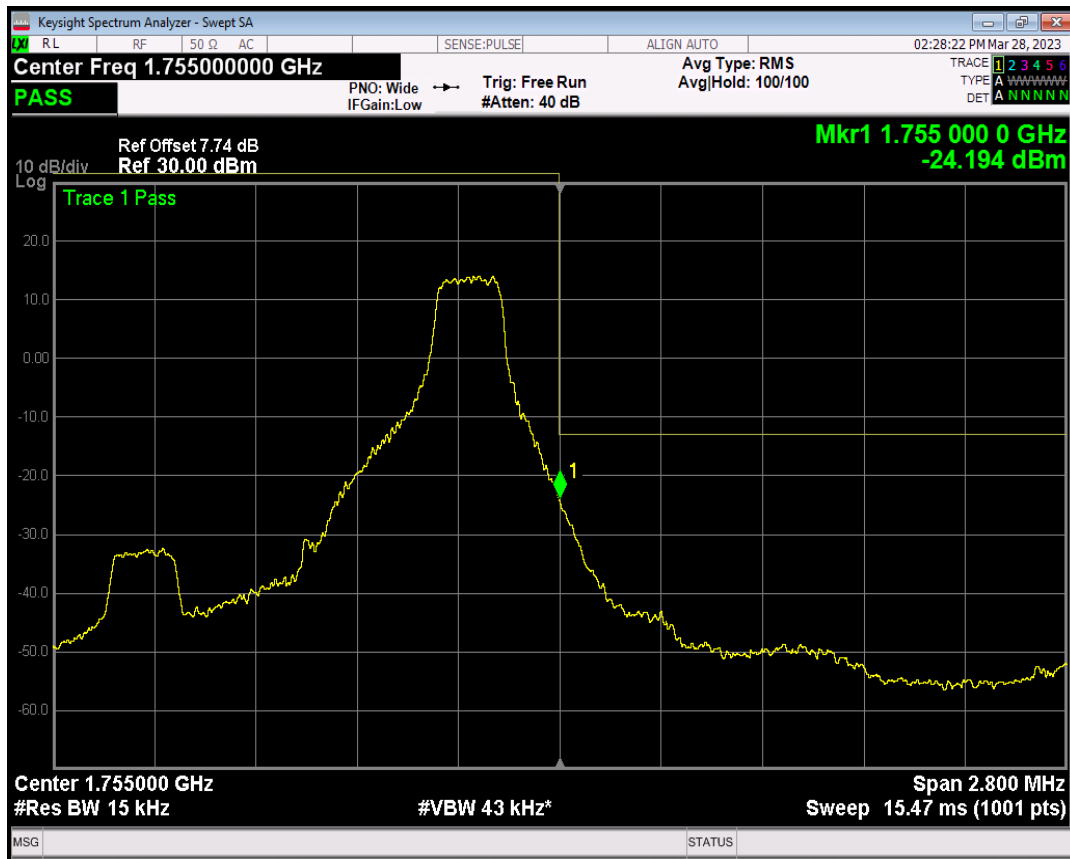
Band4 QPSK BW=1.4MHz Channel=20393 RB Size=6 Position=#0
