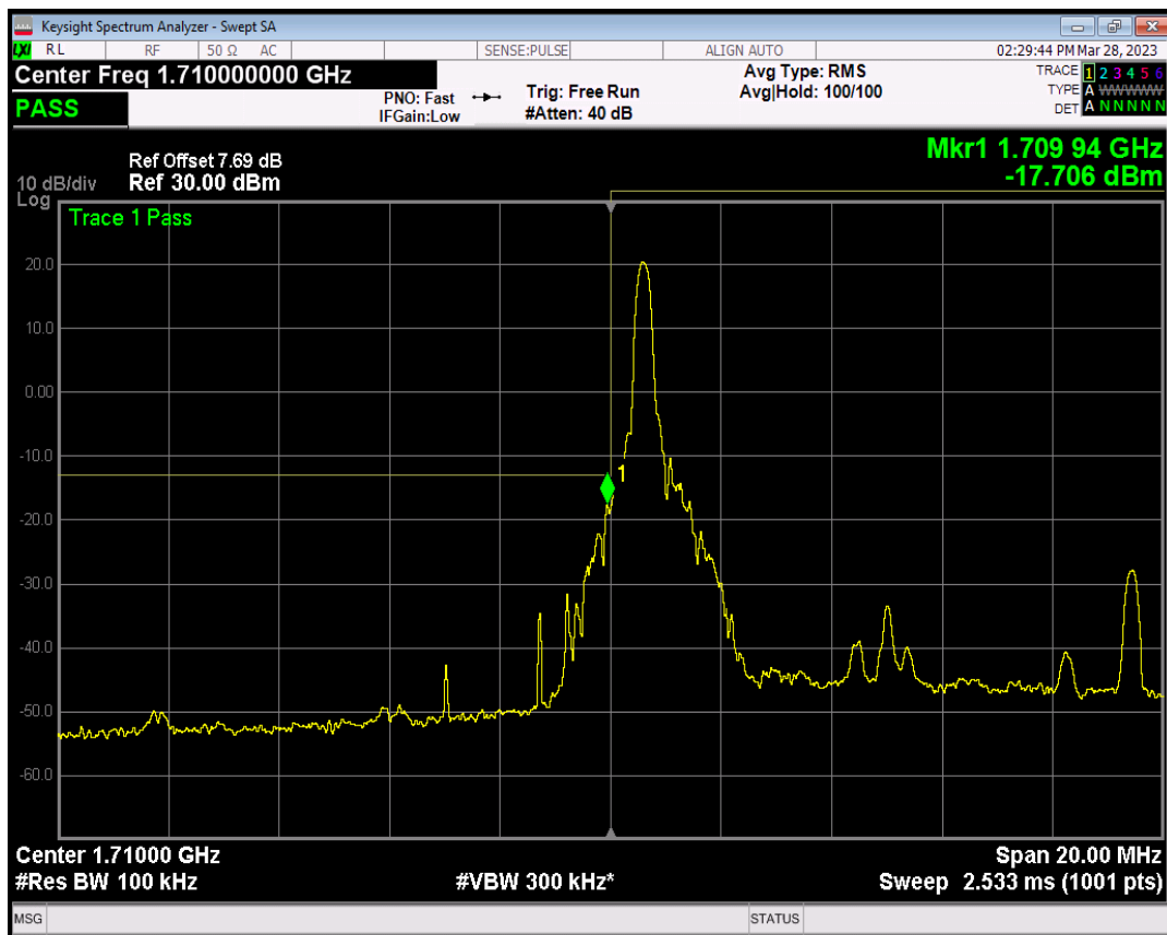
Band4 QPSK BW=10MHz Channel=20000 RB Size=1 Position=#Max
