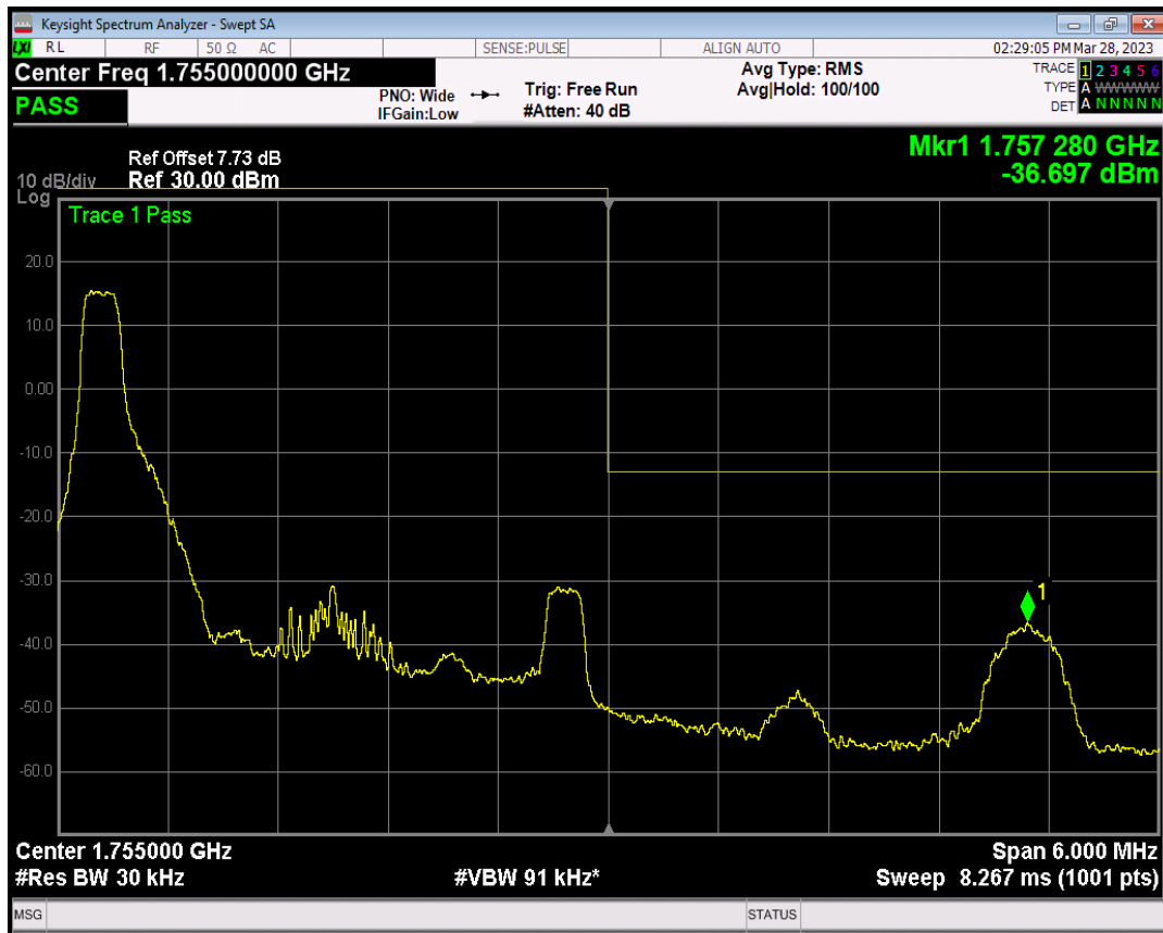
Band4 QAM16 BW=3MHz Channel=20385 RB Size=1 Position=#Max
