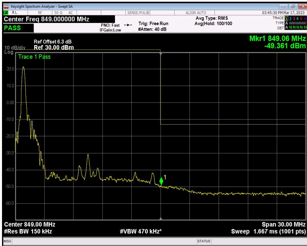
Band26(824-849) QPSK BW=15MHz Channel=26965 RB Size=1 Position=#Max
