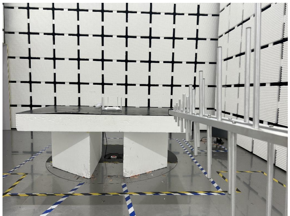
Radiation Emission Test Setup (30MHz to 1GHz)
