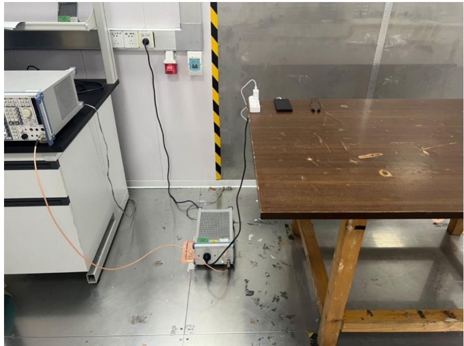
Conducted Emission Test Setup
