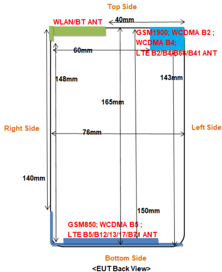
Block Diagram for EUT Antenna Position
