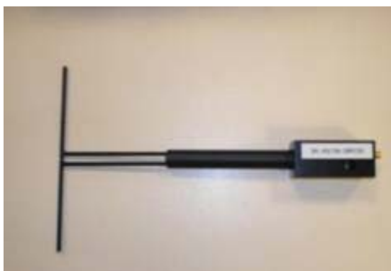
Figure 1 – MVG COMOSAR Validation Dipole
