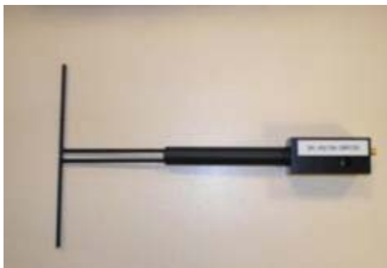
Figure 1 – MVG COMOSAR Validation Dipole
