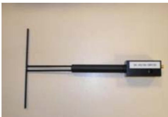
Figure 1 – MVG COMOSAR Validation Dipole
