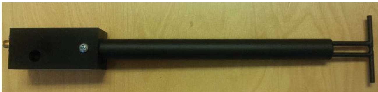
Figure 1 – MVG COMOSAR Validation Dipole
