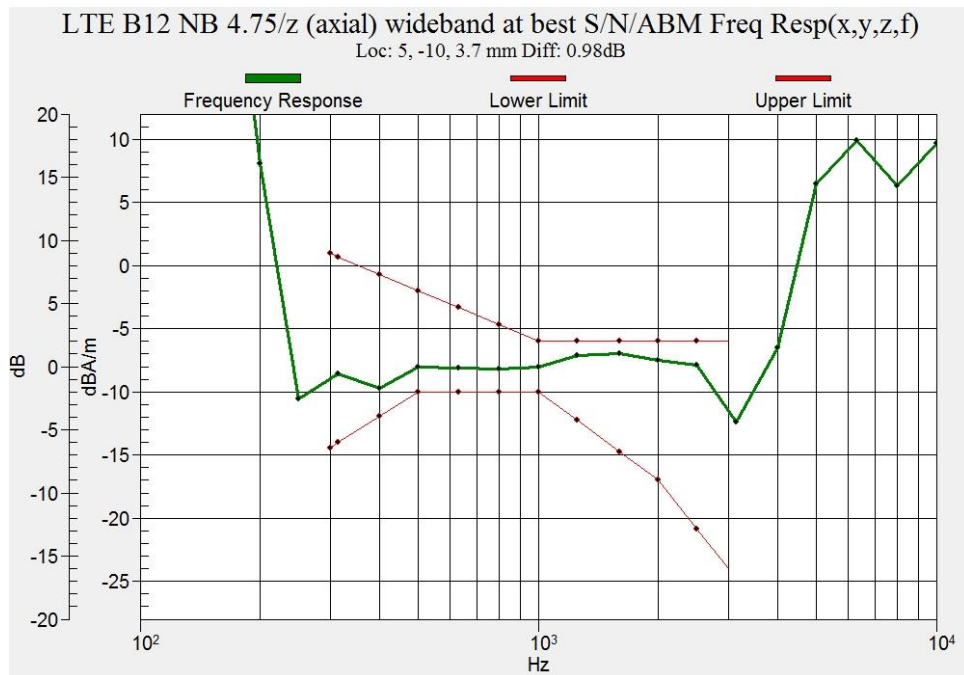
Figure B.9 Frequency Response of LTE Band 12
