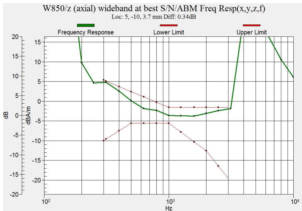
Figure B.5 Frequency Response of WCDMA Band 5
