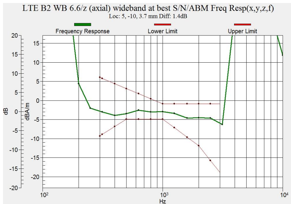
Figure B.6 Frequency Response of LTE Band 2
