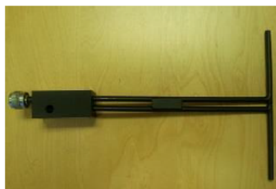
Figure 1 – MVG COMOSAR Validation Dipole
