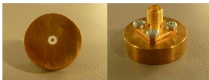
Figure 1 – MVG LIMESAR Dielectric Probe
