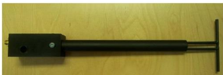
Figure 1 – MVG COMOSAR Validation Dipole
