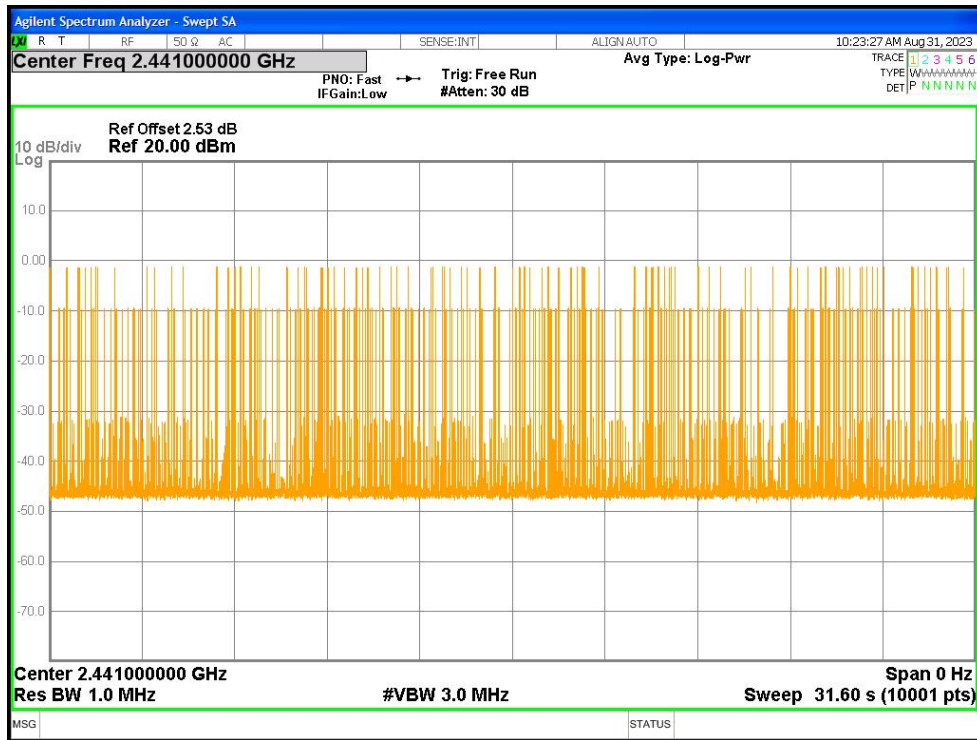
Dwell NVNT 2-DH1 2441MHz Ant1 One Burst
