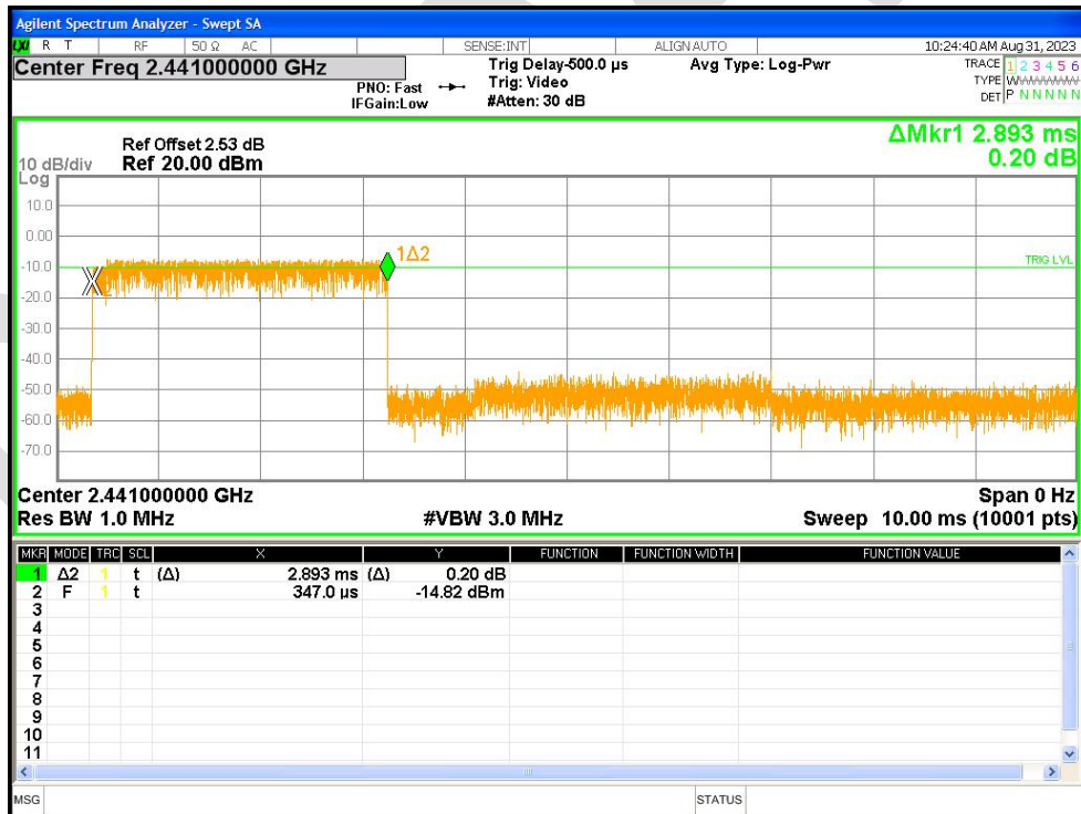
Dwell NVNT 3-DH5 2441MHz Ant1 Accumulated
