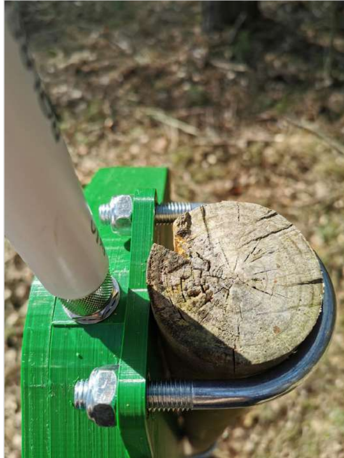
Attaching a Border Gateway to a pole using a clamp
