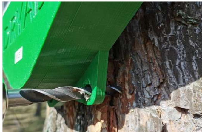
Drill the bottom two holes
