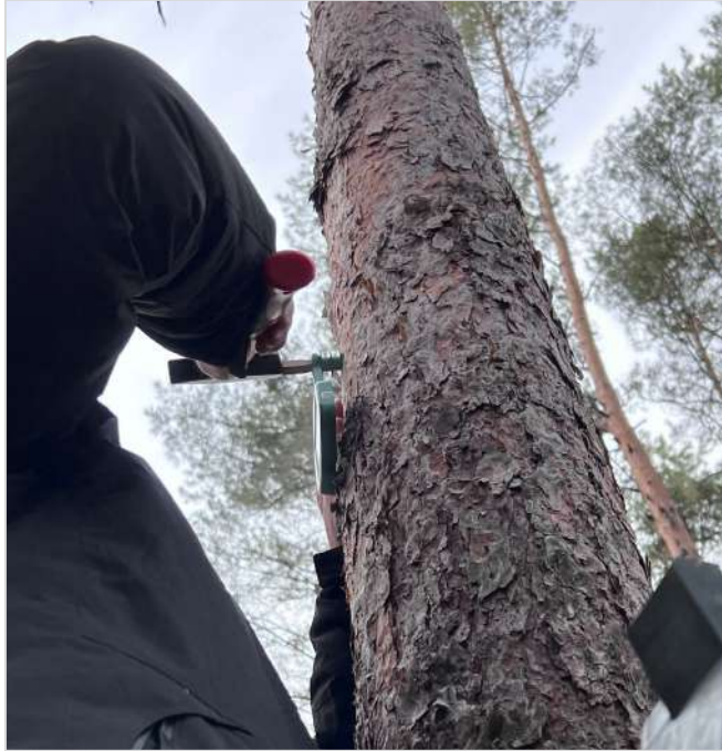
Hammer in treenail through sensor and spacer
