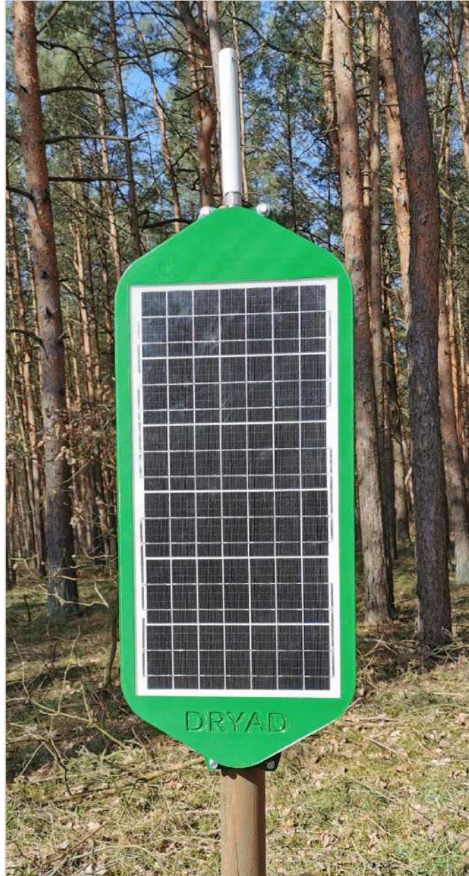
Mesh Gateway deployed on pole
