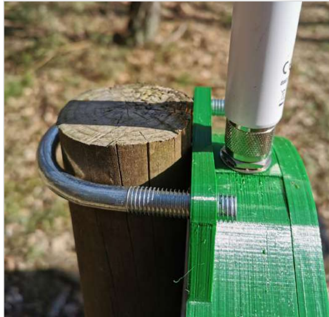
Arrange clamps around pole
