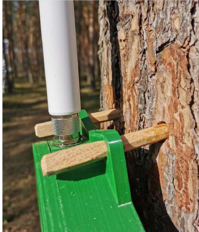
Mesh Gateway attached at the top
