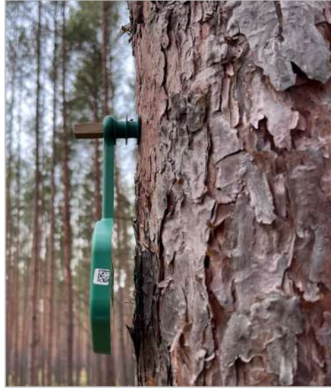
Attached sensor using tree nail
