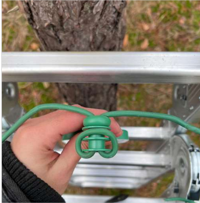
Insert crop wire through sensor and spacer
