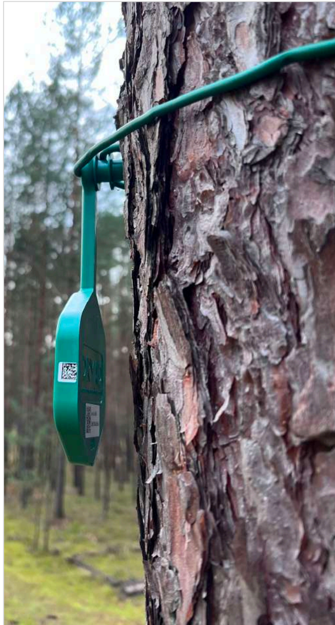
Sensor attached with crop wire
