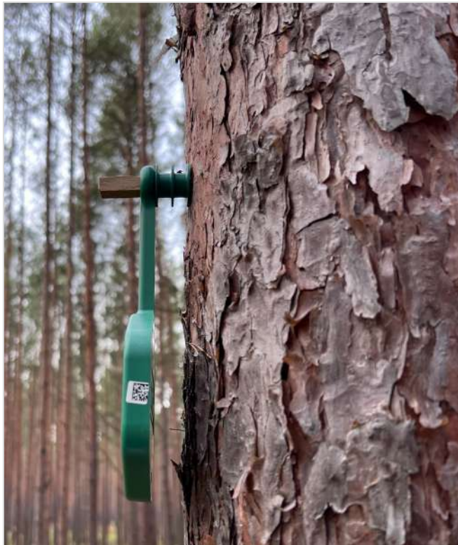
Sensor attached with treenail and spacer
