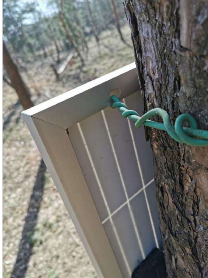
Solar panel attached using crop wire
