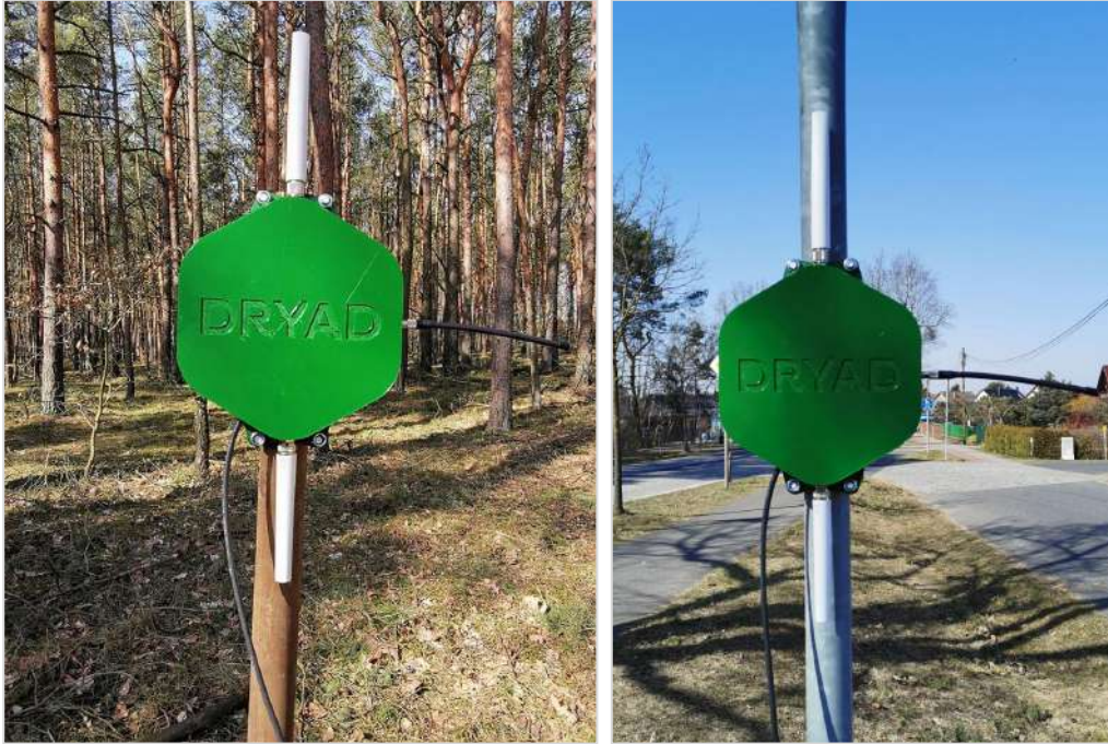
Border Gateway deployed on a pole
