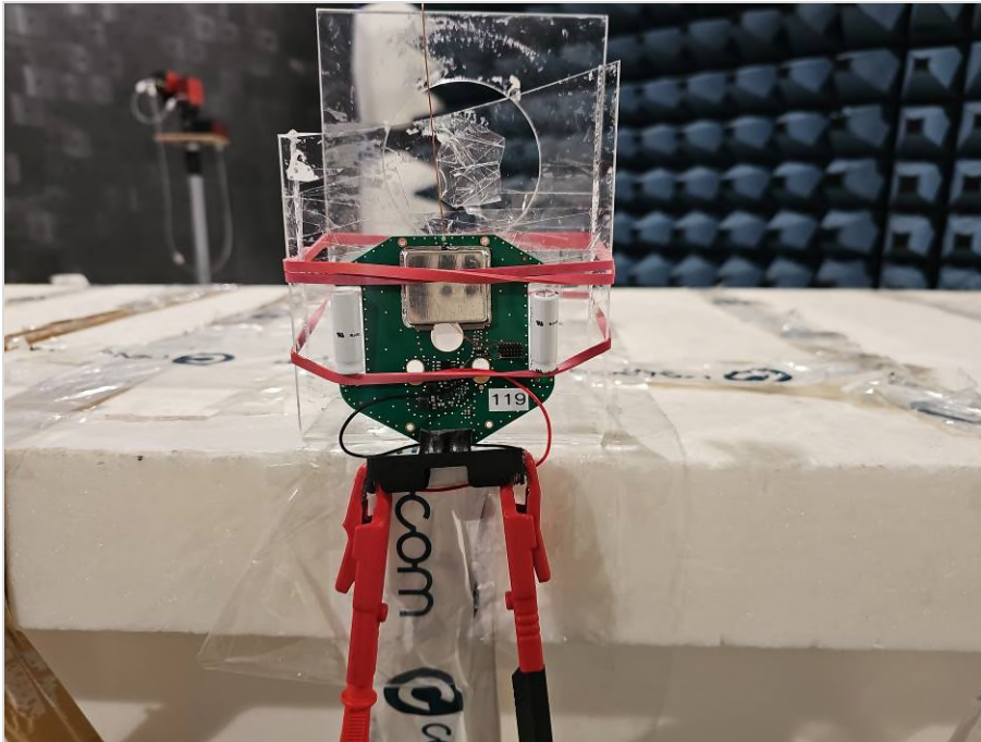
Photograph 7: EUT test setup in the semi anechoic chamber f > 30 MHz, close up view, standing
