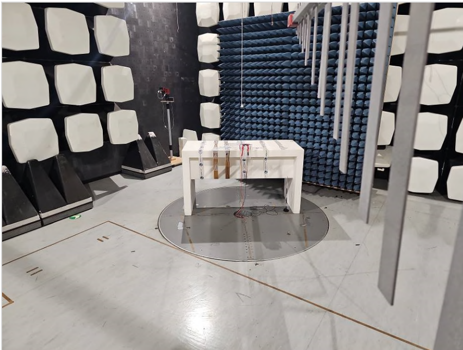
Photograph 10: EUT test setup in the semi anechoic chamber f > 30 MHz, overview, lying
