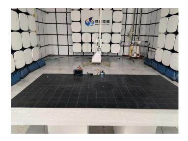
Radiated Spurious Emissions Test Frequency From 30MHz-1000MHz
