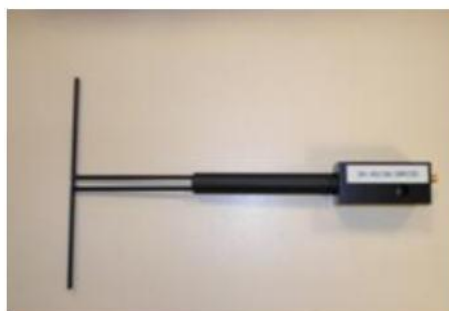
Figure 1 – Satimo COMOSAR Validation Dipole
