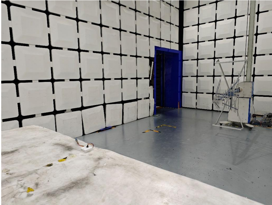
Description: RF Radiated Emission Test Setup for 30MHz ~ 1GHz (Mode1)
