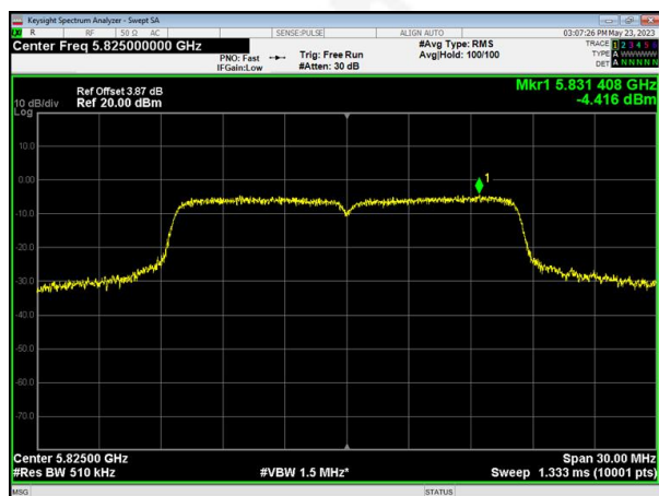
(802.11a) PSD plot on channel 165
