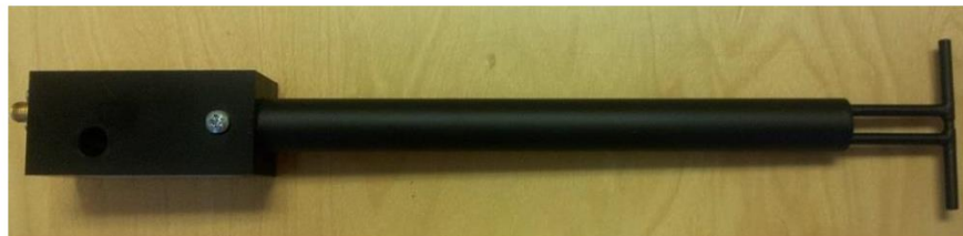
Figure 1 – MVG COMOSAR Validation Dipole
