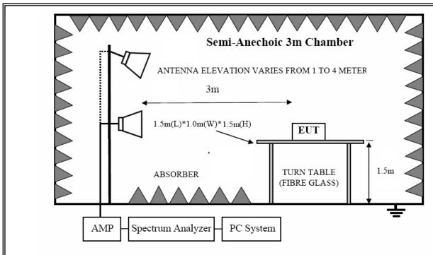
Note: For harmonic emissions test a appropriate high pass filter was inserted in the input port of AMP.
