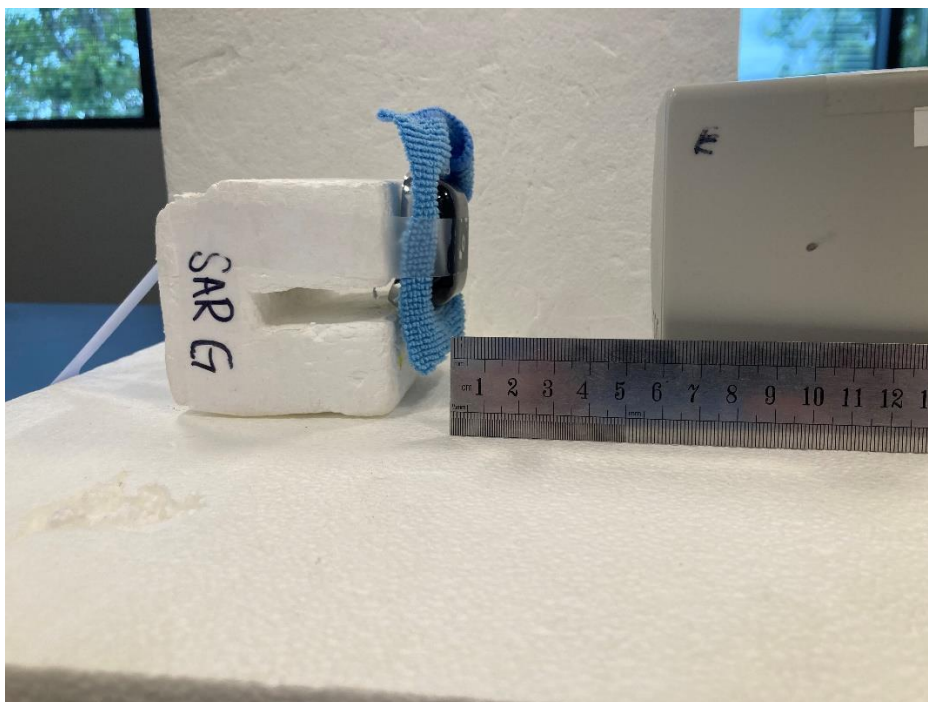
Figure 4 – Test distance 10 cm from probe center
