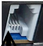
RJ11 4P4C interface(RS232 UART)
