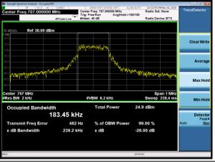
NB-IOT Band 85 QPSK 15kHz 1@0 CH-High
