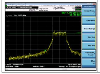
NB-IOT Band 4 QPSK 15kHz 12@0 CH-High
