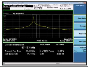
NB-IOT Band 71 QPSK 15kHz 1@0 CH-High
