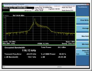
NB-IOT Band 85 QPSK 15kHz 12@0 CH-Middle
