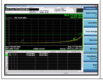
NB-IOT Band 13 QPSK 3.75kHz (793MHz ~805MHz)
