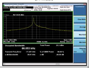
NB-IOT Band 71 QPSK 15kHz 1@0 CH-Middle
