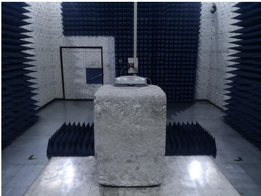
RADIATED EMISSION TEST SETUP ABOVE 1GHz
