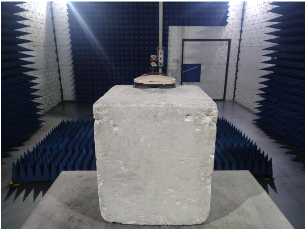
RADIATED EMISSION TEST SETUP ABOVE 1GHz
