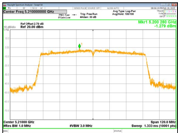
(802.11ax80) PSD plot on channel 42
