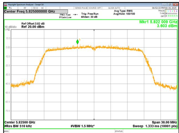
(802.11n20) PSD plot on channel 165
