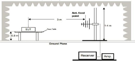
3. Radiated Emission Test-Up Frequency Above 1GHz
