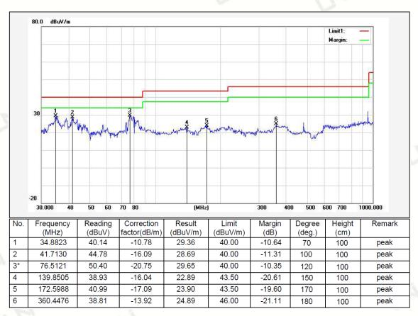
Remark: Result = Reading Level+ Factor, Margin= Result - Limit Factor=Ant. Factor + Cable Loss - Pre-amplifier
