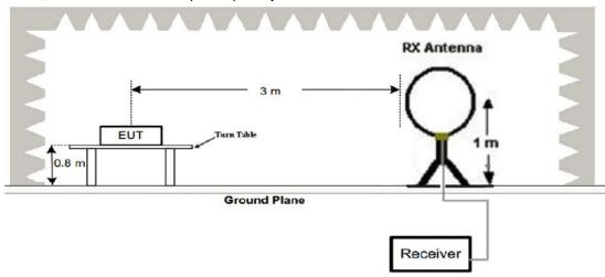
2. Radiated Emission Test-Up Frequency 30MHz~1GHz
