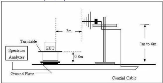
(C) Radiated Emission Test-Up Frequency Above 1GHz
