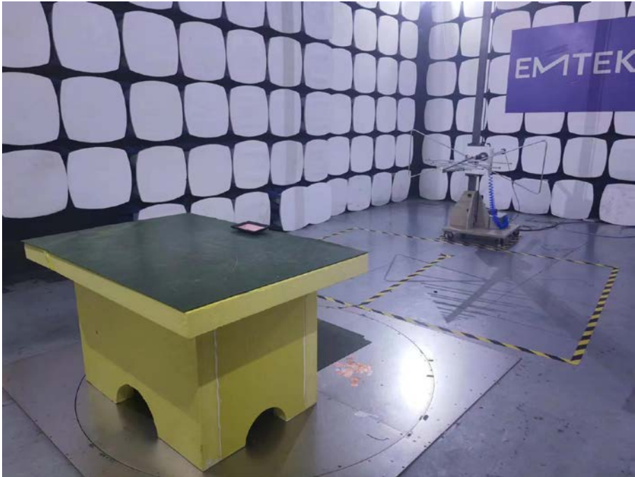
Spurious Emission Test Setup (Below 1GHz)
