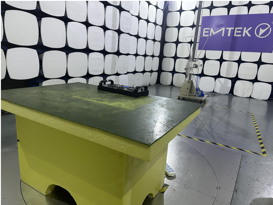
Spurious Emission Test Setup (Above 1GHz)
