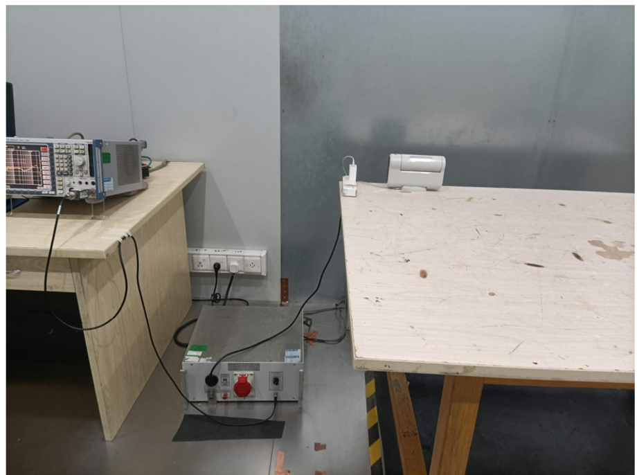
Conducted Emission Test Setup
