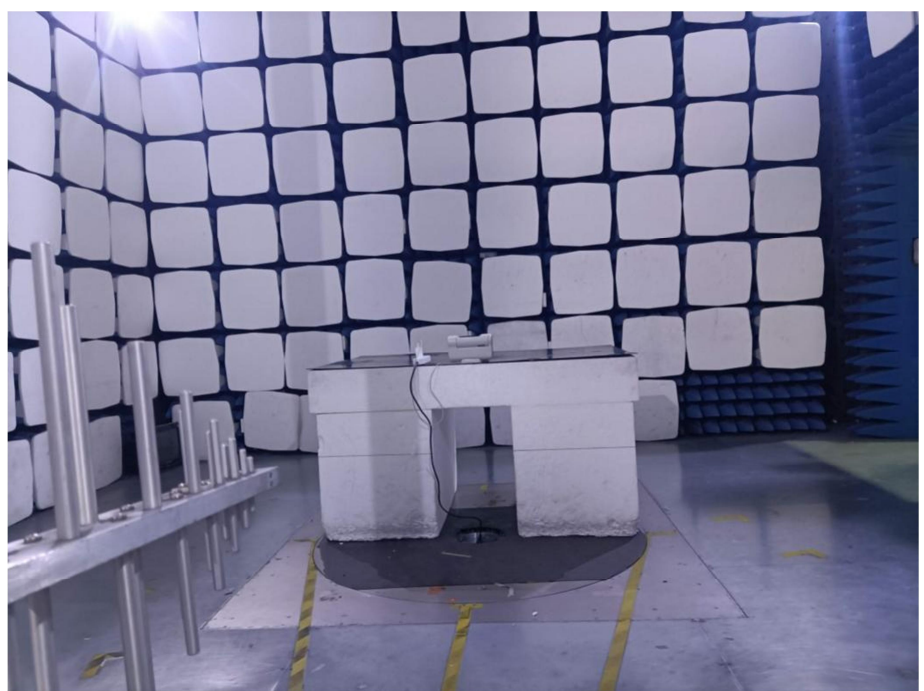
Radiation Emission Test Setup (30MHz to 1GHz)
