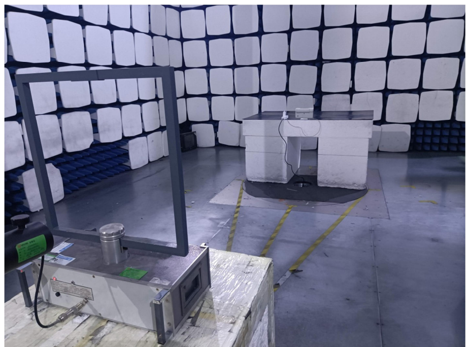
Radiation Emission Test Setup (Below 30MHz)
