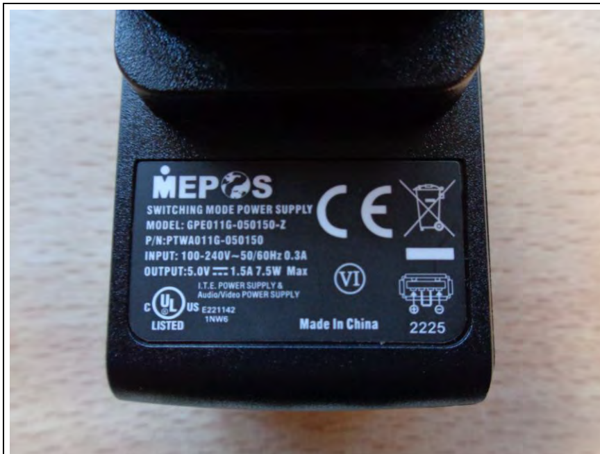
Marking Label of Power Supply
