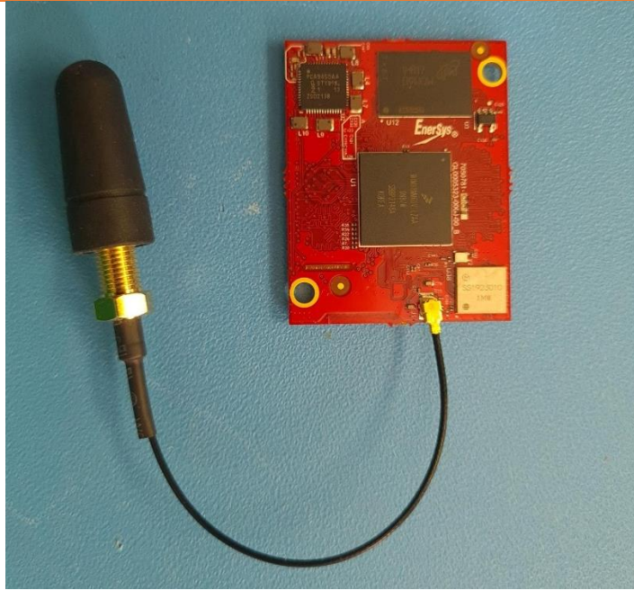
Module shown with antenna Abracon PRO-EX-347 attached with support cable
