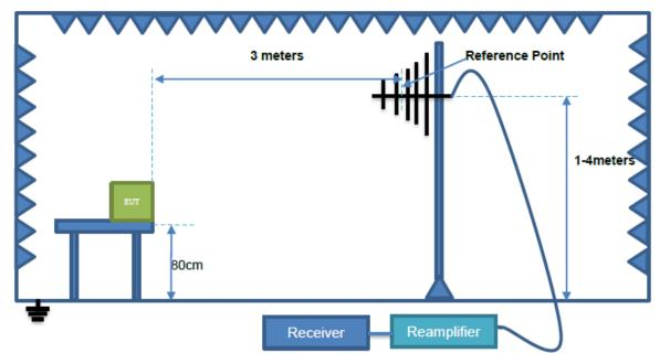
Radiation Test (30MHz - 1GHz)
