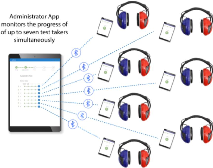
Figure 3.2: *Audhere app*. Test administrator can connect wirelessly to the test taker tablets for live progress monitoring. Maximize efficiency by testing up to seven individuals simultaneously.
