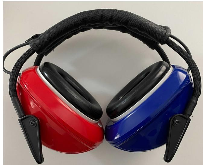
Looking closely through the black cloth inside the blue (left) ear cup, flashing blue lights should be visible after the headset has booted up and is ready for operation.
