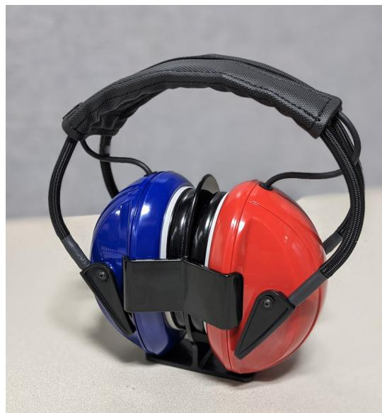
Figure 4.1: *WAHTS on Calibration Check Fixture*. To place the WAHTS in the calibration fixture, hold the WAHTS above the fixture with the ear cushions almost touching. Gently slide the WAHTS vertically down into the fixture.
