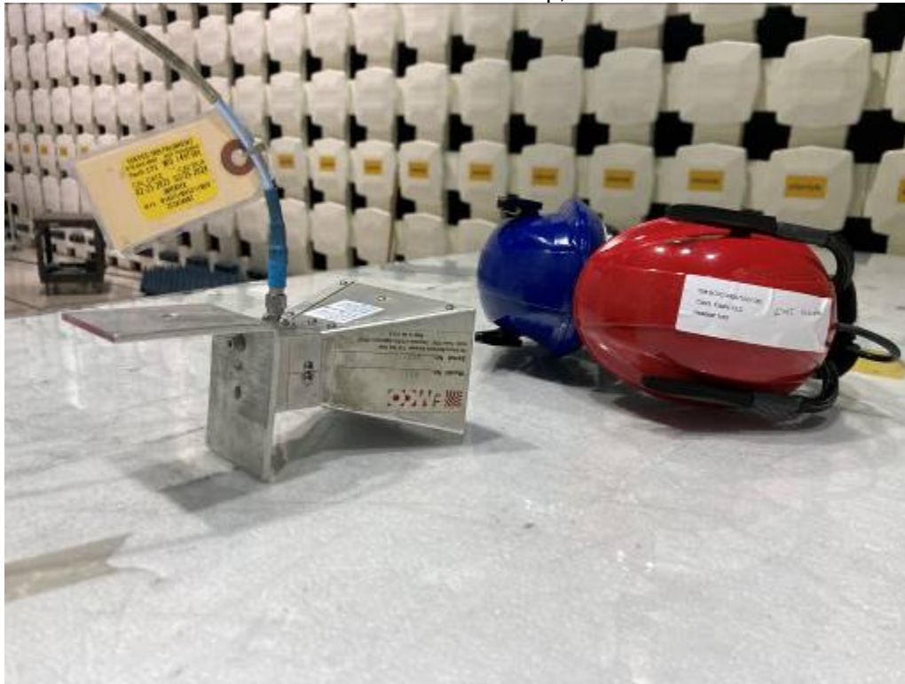
Radiated Emissions Test Setup, 18-25 GHz
