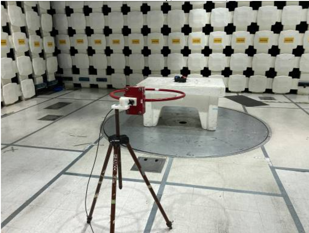
Radiated Emissions Test Setup, 9 kHz-30 MHz, Y-Axis
