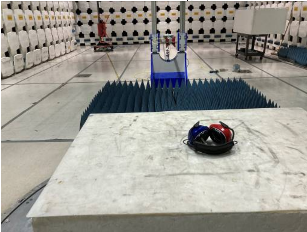
Radiated Emissions Test Setup, 1-13 GHz
