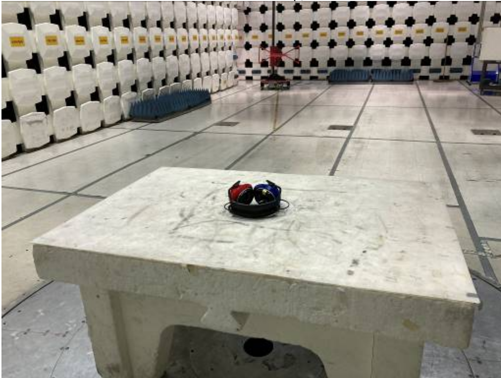
Radiated Emissions Test Setup, 30-1000 MHz
