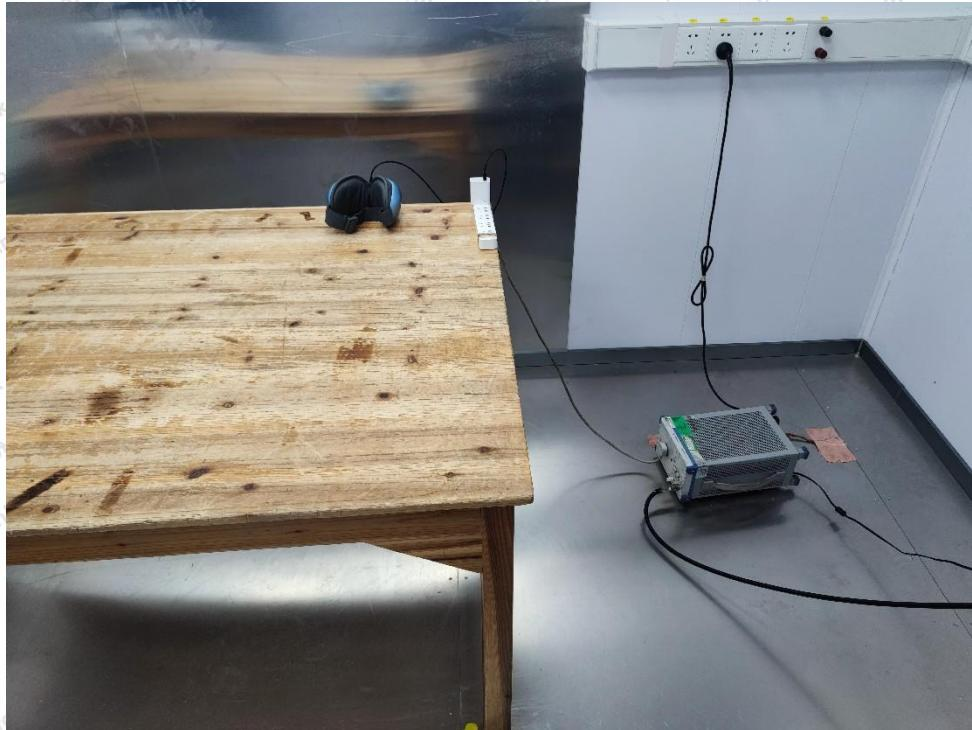
**Photo of Radiation Emission Test**
