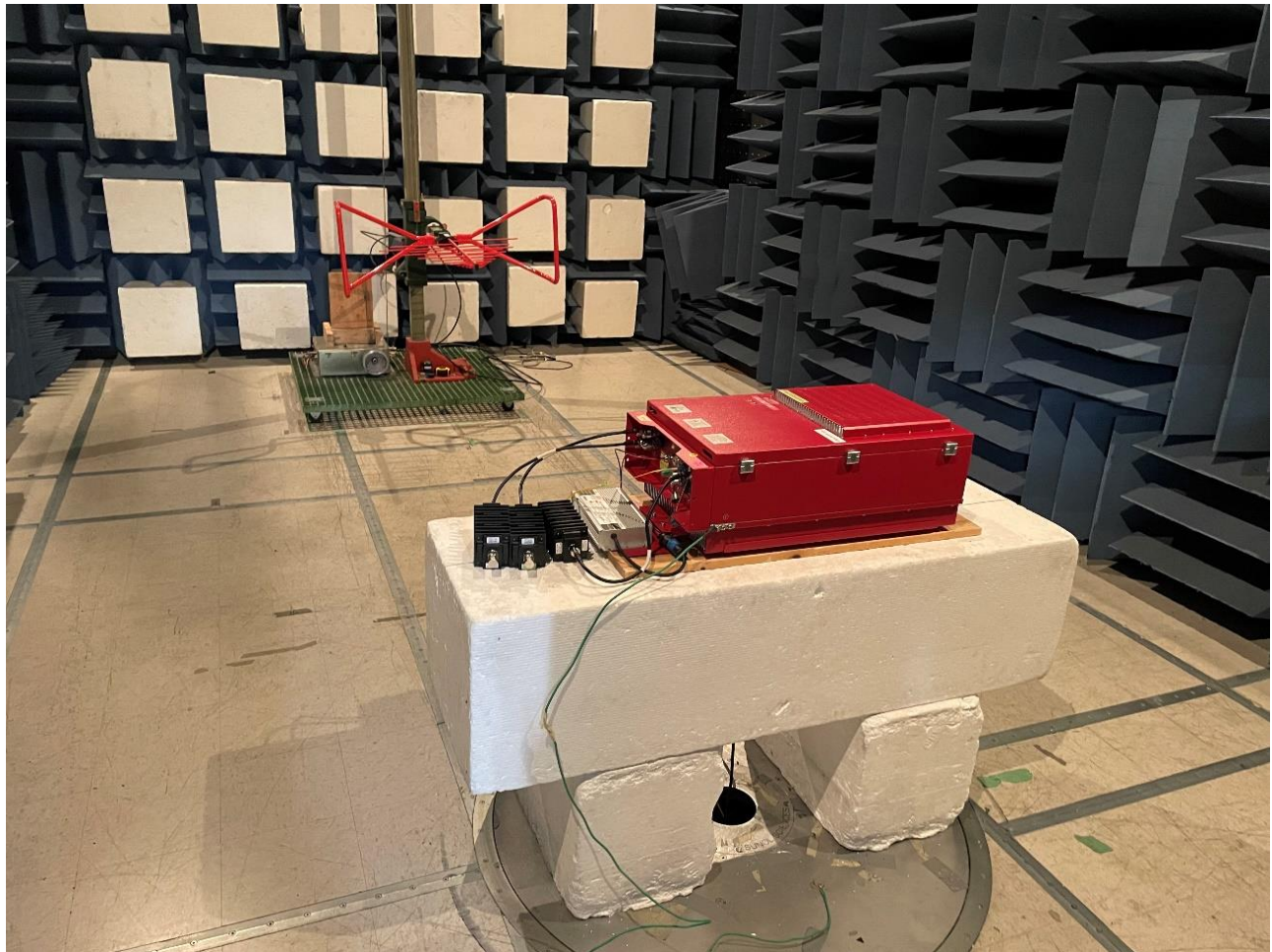
Figure 2: Radiated Emissions (Below 1GHz) Test Setup
