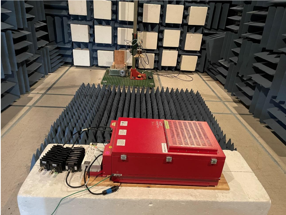
Figure 3: Radiated Emissions (Above 1GHz) Test Setup
