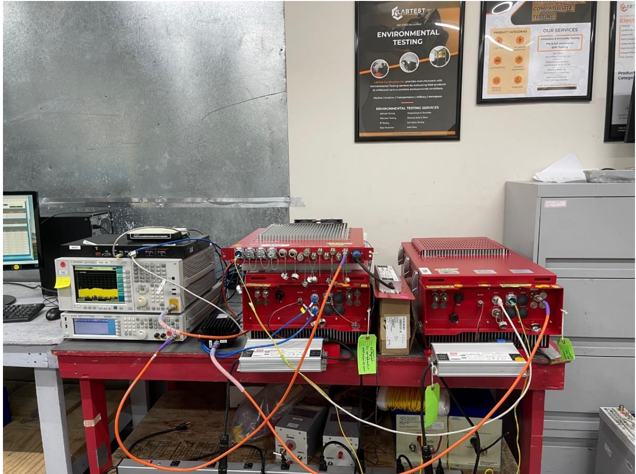
Figure 1: RF Conductive Emissions Test Setup
