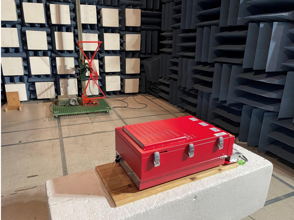
Figure 2: Radiated Emissions (Below 1GHz) Test Setup
