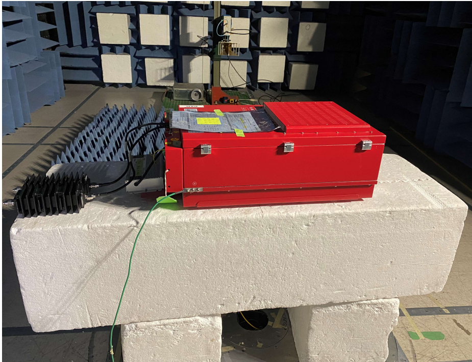
Figure 3: Radiated Emissions (Above 1GHz) Emissions Test Setup
