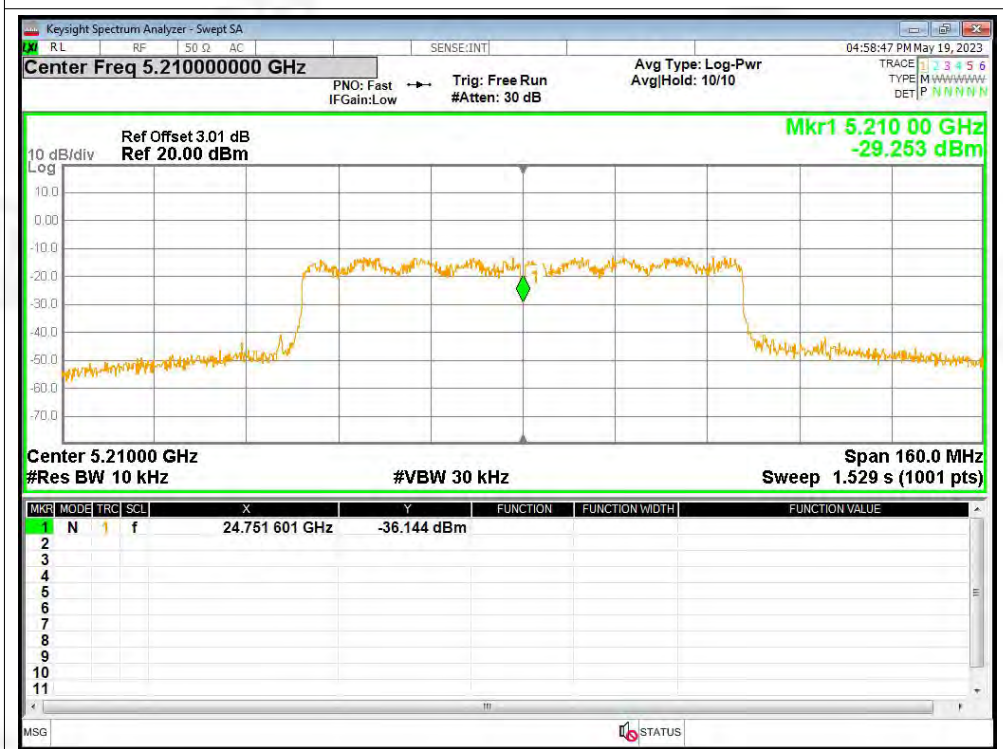
Freq. Stability NVNT ac80 5210MHz Ant1
