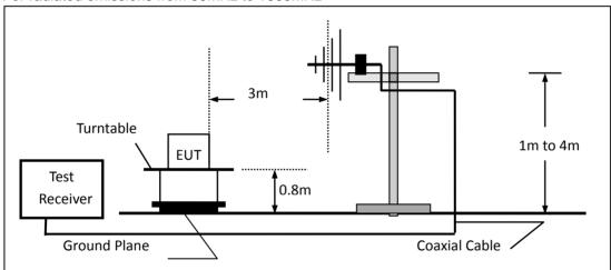
(c) For radiated emissions above 1000MHz
