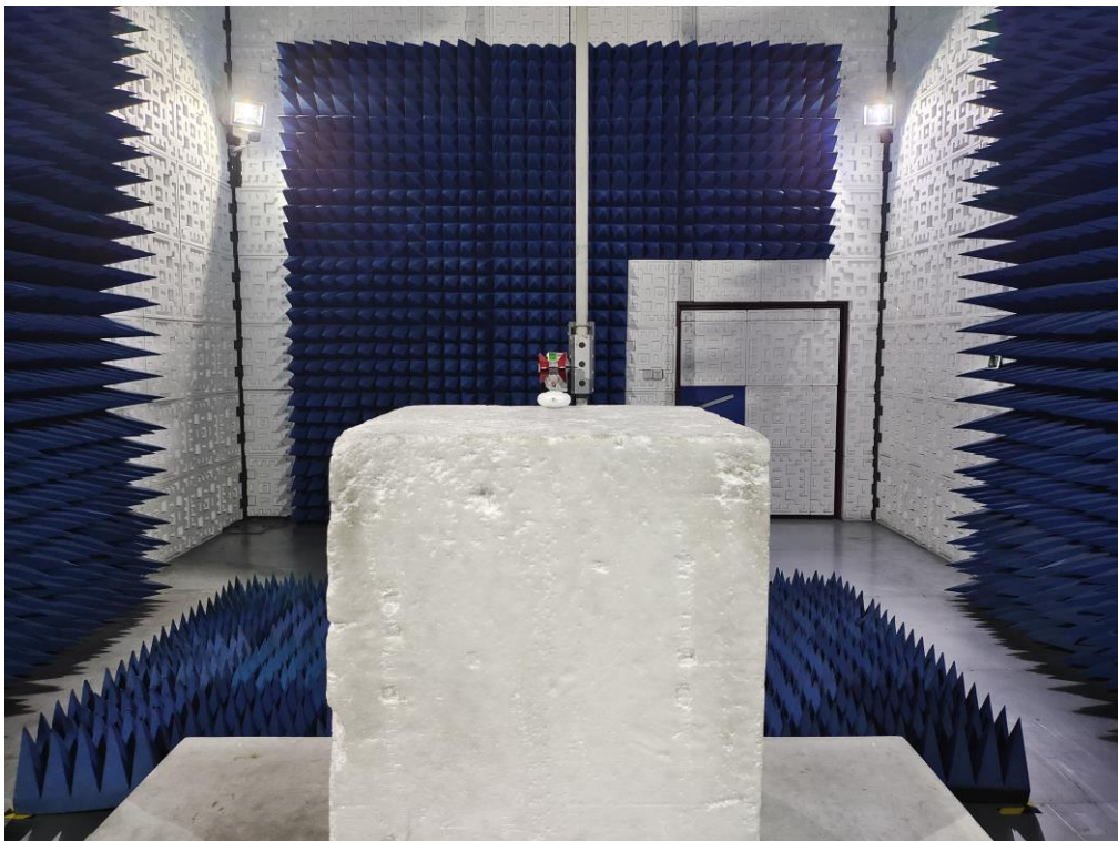
RADIATED EMISSION TEST SETUP ABOVE 1GHz
