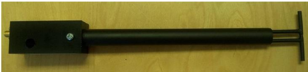
Figure 1 – MVG COMOSAR Validation Dipole
