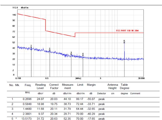
Note:1. \*:Maximum data; x:Over limit; !:over margin. 2.Measurement=Reading Level+Correct Factor; Correct Factor=Antenna Factor+Cable Loss.
