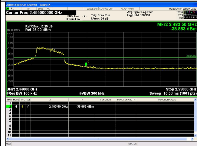
Out Of Band Emission IEEE 802.11g_Channel 11_20MHz_Antenna 0
