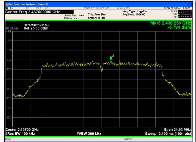
In-Band Reference Level IEEE 802.11g_Channel 6_20MHz_Antenna 0
