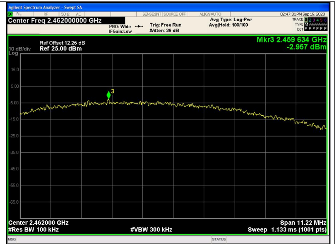
In-Band Reference Level IEEE 802.11b_Channel 11_20MHz_Antenna 0
