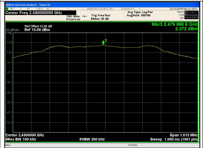
In-Band Reference Level LE_Channel 39
