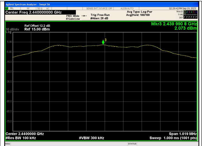
In-Band Reference Level LE_Channel 19
