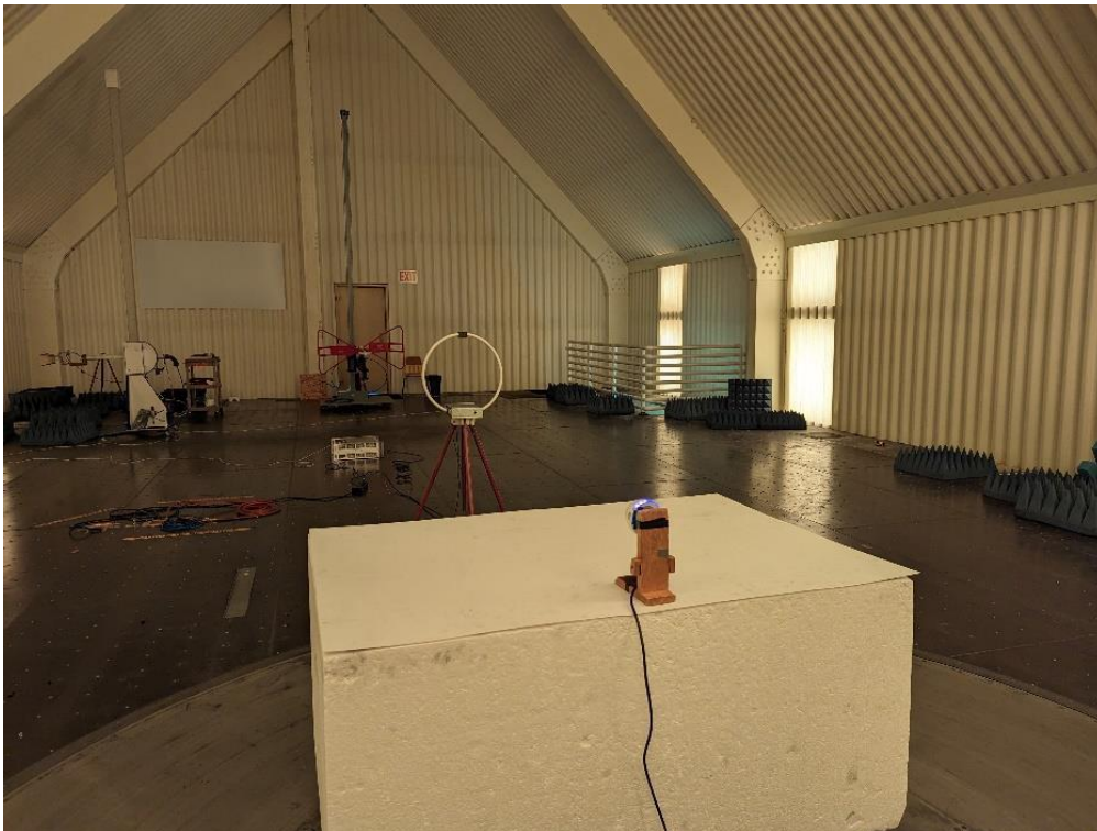
Photograph 4: Back View Radiated Emissions Worst Case – Below 30 MHz Configuration
