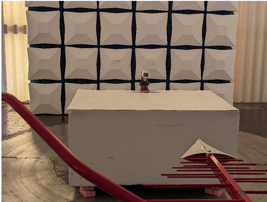
Photograph 1: Front View Radiated Emissions, 30 to 1000 MHz Worst Case Configuration
