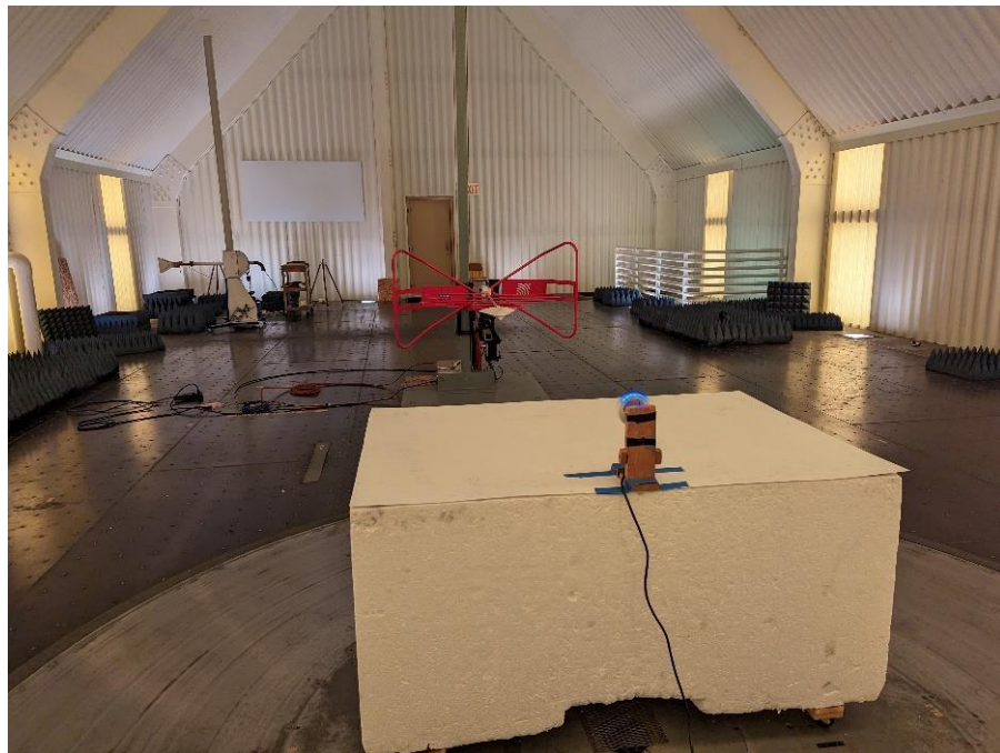
Photograph 2: Back View Radiated Emissions, 30 to 1000 MHz Worst Case Configuration
