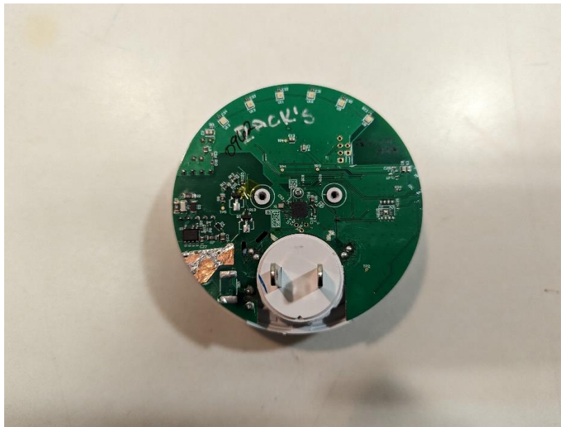
Photograph 10: Internal View of the EUT with 13.56MHz Transmitter Circuitry
