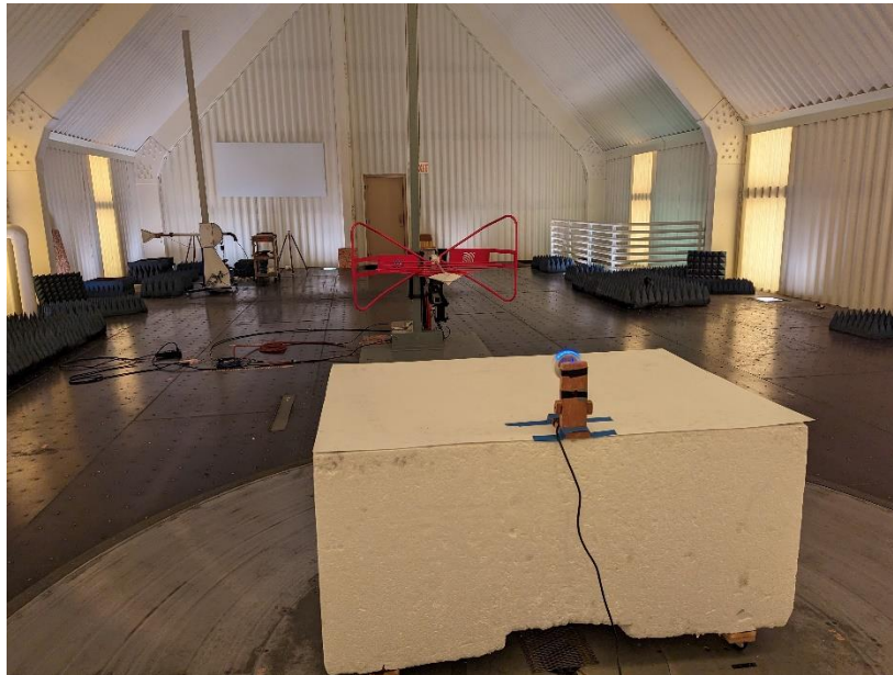
Photograph 4: Back View Radiated Emissions Worst-Case Configuration
