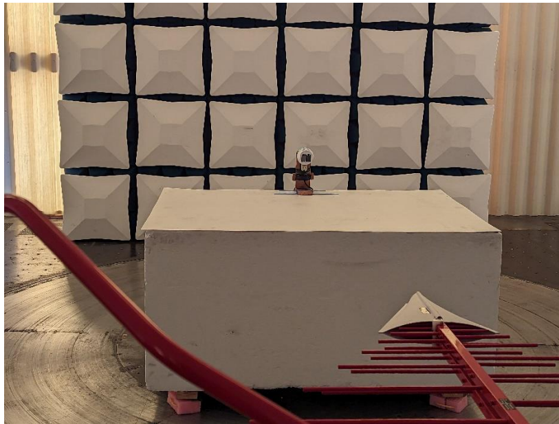
Photograph 3: Front View Radiated Emissions Worst-Case Configuration
