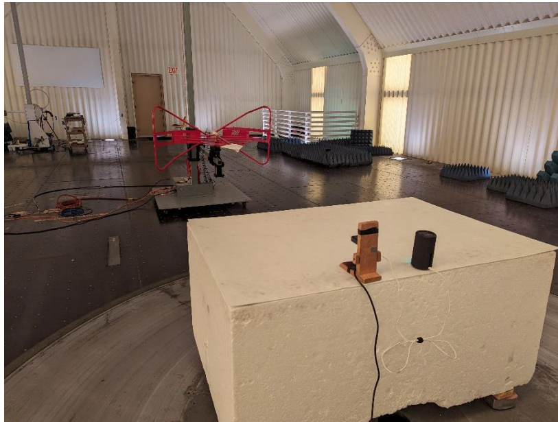
Photograph 4: Back View Radiated Emissions Worst-Case Configuration – Frequencies 30-1000MHz
