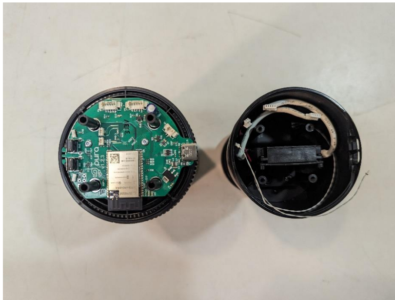
Photograph 16: Placement of PCB in Enclosure with Cabling Removed
