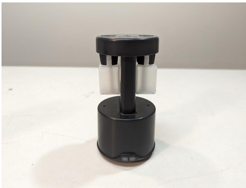
Photograph 13: EUT with Outer Cowel Removed and Scent Bottles in Place
