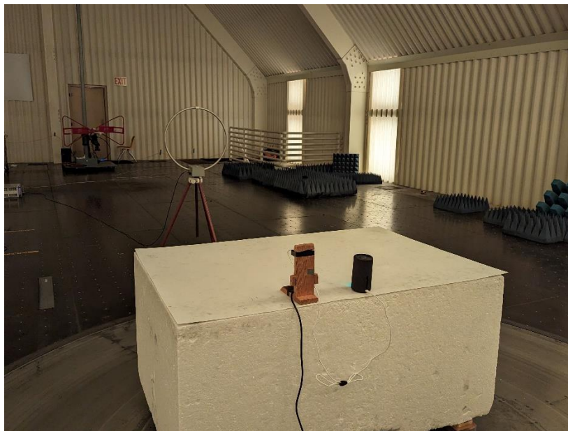
Photograph 2: Back View Radiated Emissions Worst-Case Configuration – Frequencies Below 30MHz
