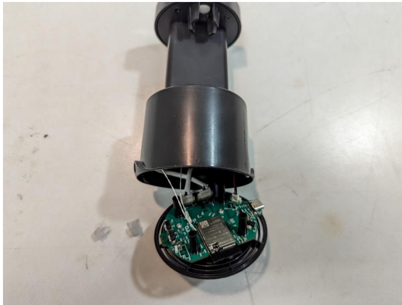
Photograph 15: Placement of PCB in Enclosure
