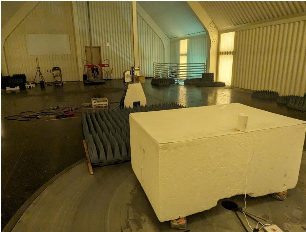
Photograph 6: Back View Radiated Emissions above 1000 MHz Worst Case Configuration
