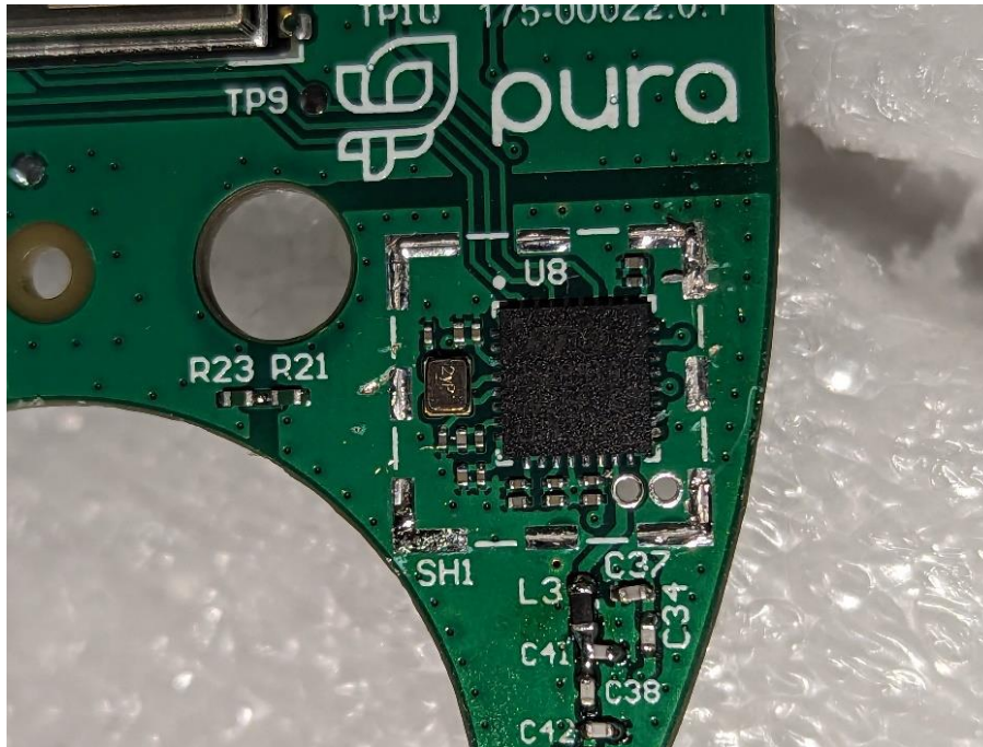
Photograph 3 – Close-up View of the RF Circuitry Under the Shield
